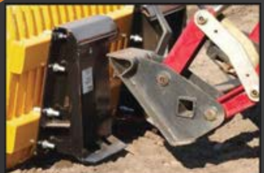
Attaching brackets are designed to respect the original manufacturer's designed angles.
