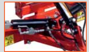
Two hydraulic cylinders with ball valves
