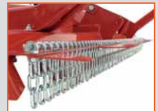
Chains provide safety from thrown objects
