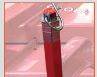
Hexagonal yokes on front tires of rear mower deck prevent slippage on slopes
