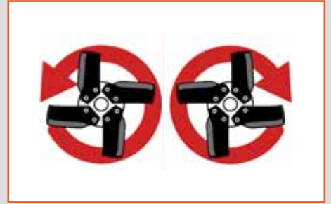
Forward or reverse tilling rotation
