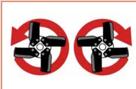
Forward or reverse tilling rotation
