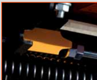
Easy to inspect and adjust belt tensioner
