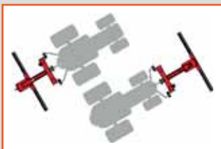
Front or rear tractor mounting
