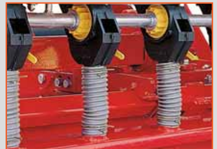
Precise seed metering cups
