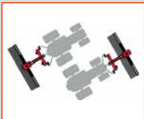
Front or rear tractor mounting
