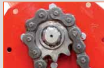
Lateral ASA 100 chain drive transmission in oil bath
