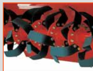
Rotor with 6 blades per flange
