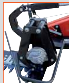
Cast aluminium connecting rods with cooling fins
