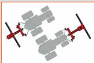
Front or rear tractor mounting
