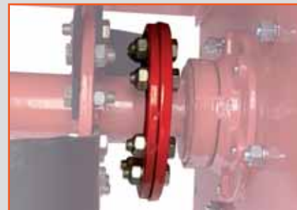
Rotor shaft with flanges for easy blade replacement
