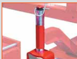
Hexagonal yokes on front tires of rear mower deck to prevent slippage on slopes
