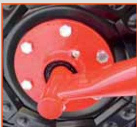
Cast steel hubs with greasable tapered bearings
