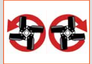
Forward or reverse tilling rotation
