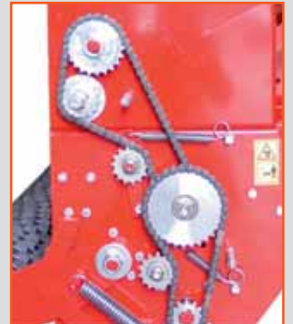
Seed distribution engaged by ASA 50 chain transmission
